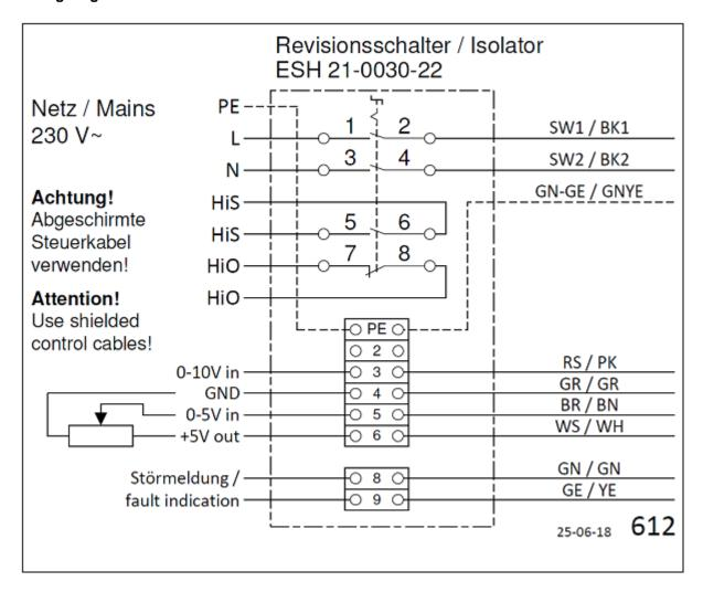
Wiring diagram for connection to: mains - service switch & VSD - motor
